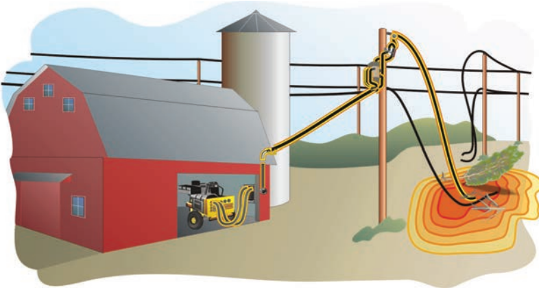
Backfeed from Generator
